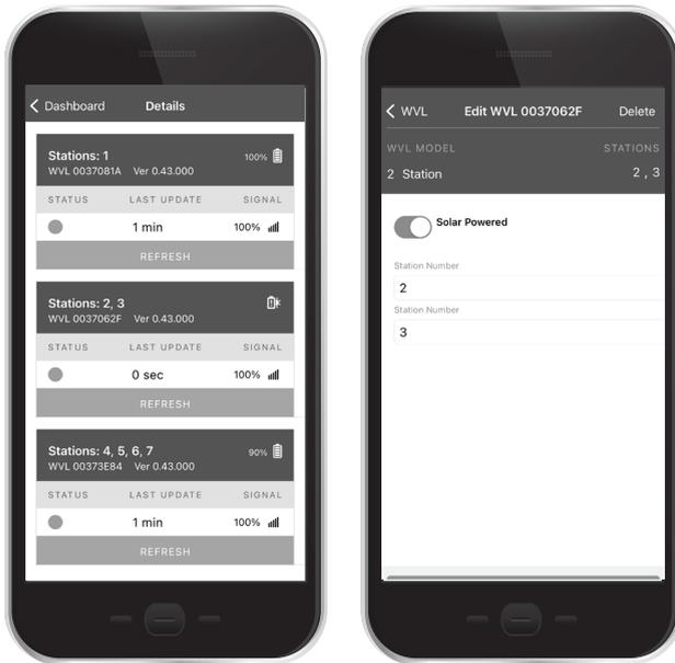
When using the Solar Panel with a Wireless Valve Link, use the Bluetooth® enabled Hunter Wireless Valve Link App to designate the Wireless Valve Link as "Solar Powered."
